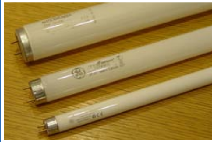
Replacing T12 fluorescent bulbs (top) with the more efficient T8 bulbs (center) can provide the same quality of light while drawing less power and reducing heat output, making the T8 a more efficient choice.
