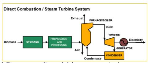
Figure 1: The most common biomass fueled power generator is a direct combustion/steam turbine system. Figure courtesy of the US Department of Energy, Energy Efficiency and Renewable Energy Program.
