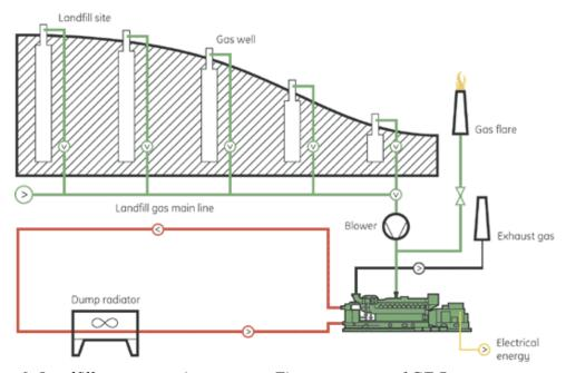
Figure 6: Landfill gas generation process. Figure courtesy of GE Power.
